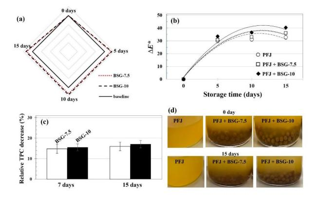
Figure 5. Storage time dependence on (a) SR of the hydrogels, (b)  $\Delta E^*$  of PFJ, (c) relative TPC decrease of the hydrogels, and (d) appearance of the PFJ.
