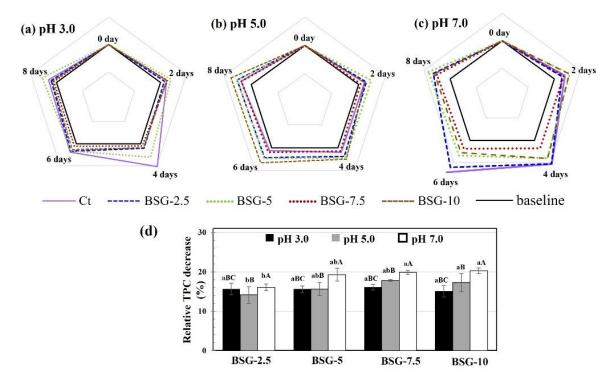
**Figure 4.** SR of hydrogels stored at pH (**a**) 3.0, (**b**) 5.0, and (**c**) 7.0 for different storage times, and (**d**) relative TPC decrease of hydrogels after 8-day storage at different pH conditions. In (**d**), different lowercase letters indicate significantly different means as affected by BSG content, and different uppercase letters indicate significantly different means as affected by pH.
